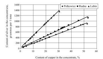
Fig. 2. The relationship between the content of silver and copper in concentrates obtained from laboratory flotation
