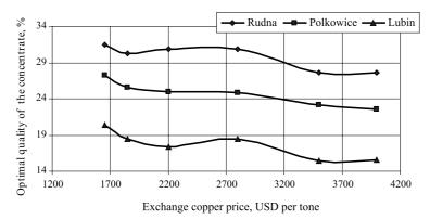
Fig. 3. The influence of copper exchange price on optimal qualities of concentrates processing in Rudna,
